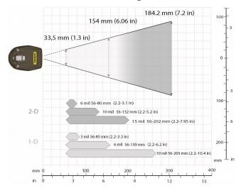
Note: The calibration distance is 143.0 mm from the nose of the lens, and the calibration tolerance is +/- 5 mm.
