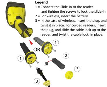
Note: Disconnect the DataMan 8600 from power or remove the battery before inserting/removing the communication modules.
